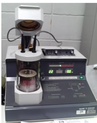
Figura 3.12 – Sputter Coater BAL-TEC SCD 050 (LNLS – Campinas).
