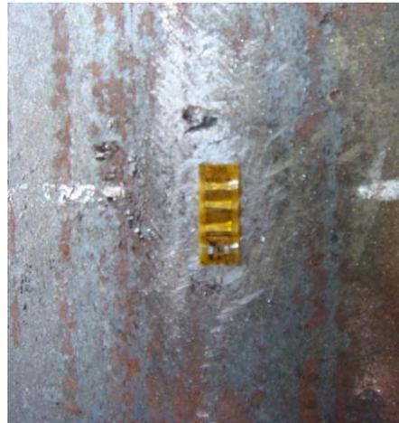
Figura 47 - Strain gage deformado
