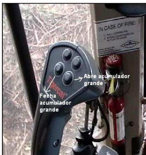
FIGURA 52- *Joystick* Esquerdo - Feller-Buncher
