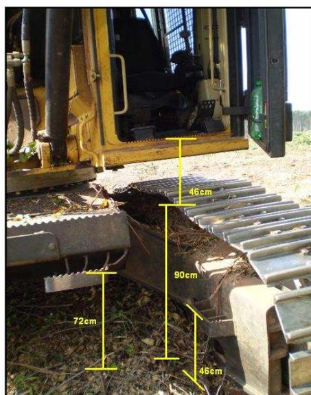
FIGURA 48 - Acesso a cabine do Feller-Buncher
