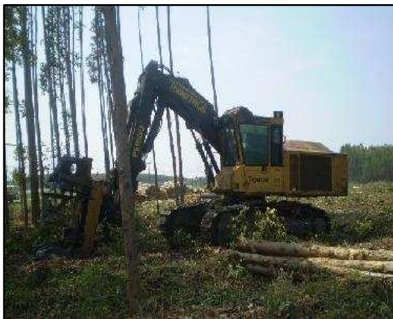
FIGURA 18 - Feller-Buncher 860 C Tigercat.
