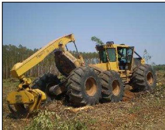
FIGURA 19 - Skidder 635 D (6x6) – Tigercat.
