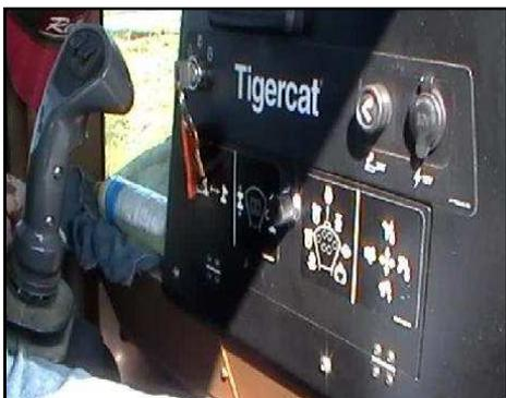
FIGURA 29 – Painel lateral – Skidder.
