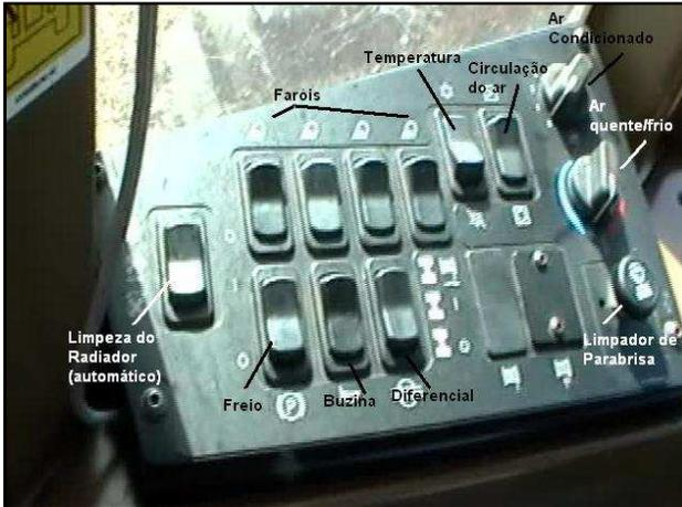
FIGURA 26 - Painel frontal Skidder 635 D
