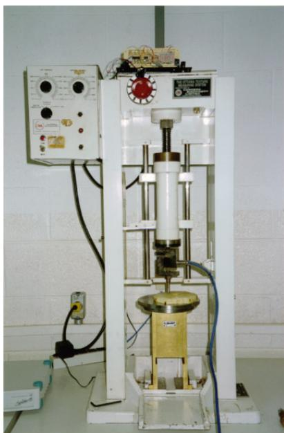
**Figura 2.** Penetrômetro The Ottawa Texture Measuring System.
