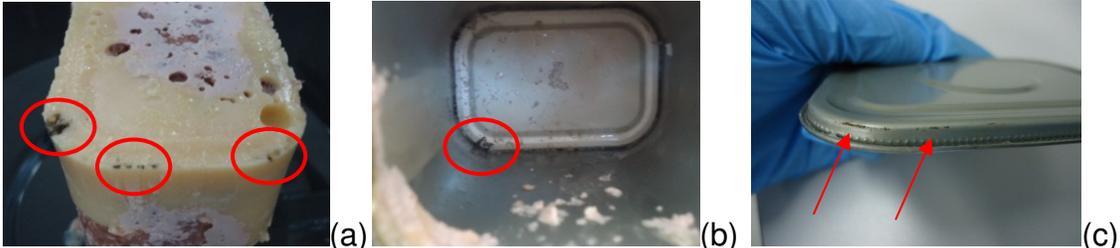
Figure 3.7. Photographs illustrating the sulphide black in the seaming position (a) and (b) and metal exposure evidenced by the application of copper sulfate (c).
