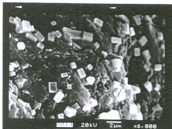
Fig. 2 Micrographs of the morphology of microcapsules submitted to immersion in a solution at pH 1: a. zero time; b. after one h; c. after two h
