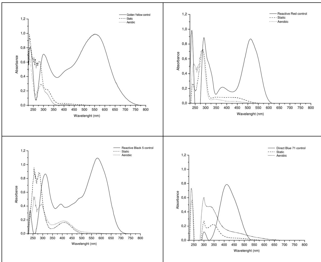
**Figure 3.** UV-vis spectra of the azo dyes before (straight line) and after microaerophilic (dashed line) and aerobic (dotted line) treatments: (A) RY107, (B) RR198, (C) RB5, (D) DB71.
