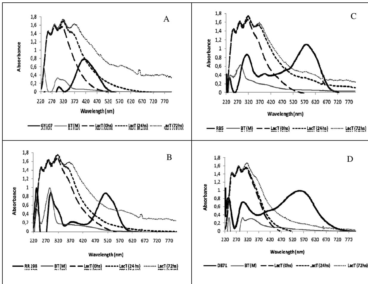
**Figure 2.** UV-Vis spectra of the azo dyes before (bold straight line) and after bacterial (straight line) and laccase (dashed and dotted line) treatments - A: RY107; B: RB5; C: RR198; D: DB71; BT (M): Bacterial treatment under microaerobic conditions; LacT: Laccase treatment after 0, 24 and 72 hs.
