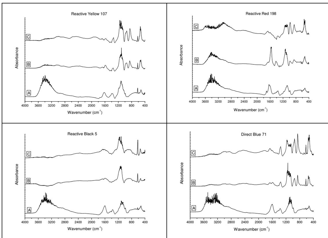
**Figure 3.** FT-IR spectra of the azo dyes before (A) and after microaerophilic (B) and aerobic (C) treatments
