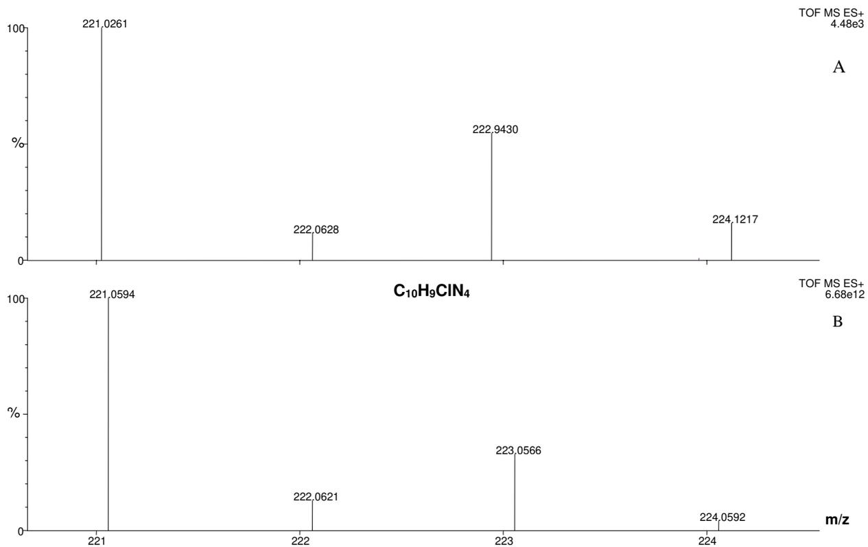
**Figure 4.** Mass spectra of the RR 198 azo dye metabolite (A) in comparison to standart 4-chloro-N-o-tolyl-1,3,5-triazin-2-amine (B).
