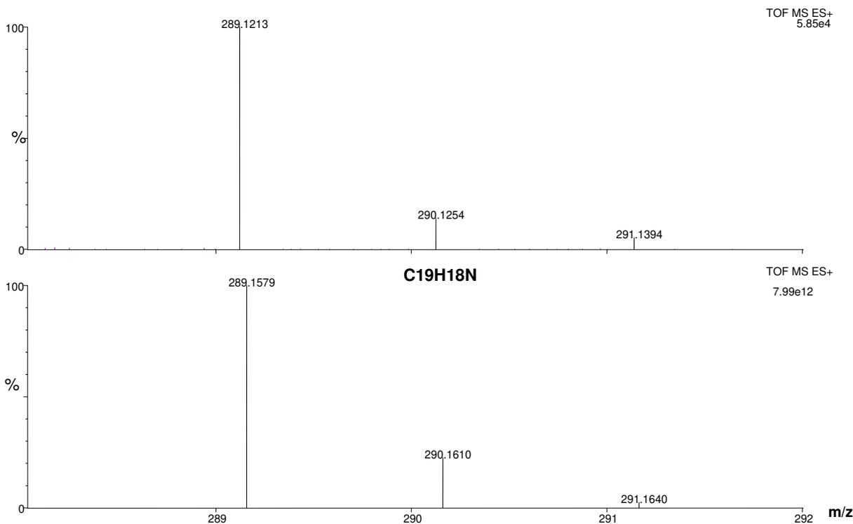
**Figure 6.** Mass spectra of the RR 198 azo dye metabolite (A) in comparison to standard 3,6-dimethyl-7-(o-tolyldiazenyl) naphthalen-1-amine (B).
