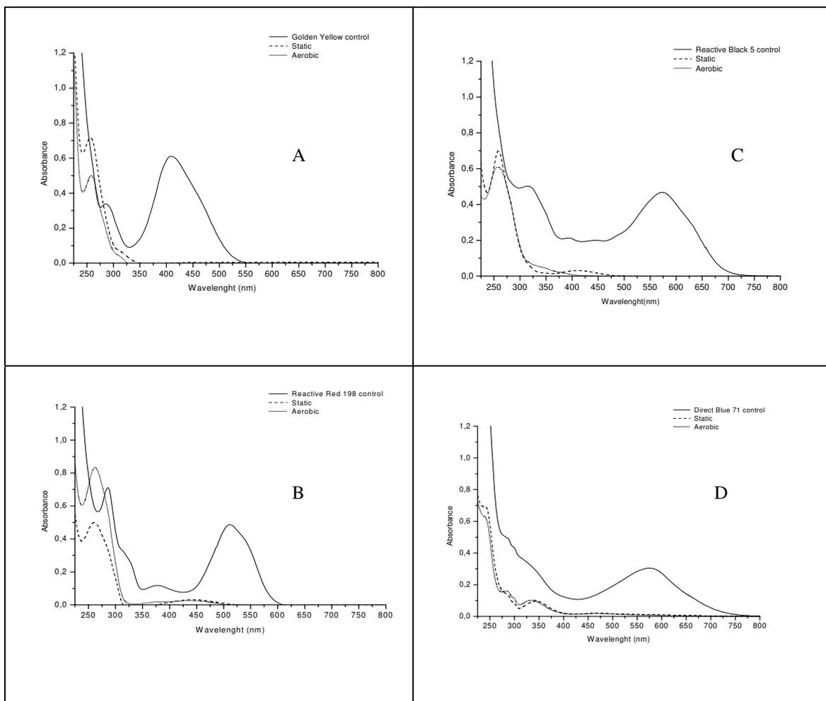
**Figure 2.** UV-Vis spectra of the azo dyes before (straight line) and after microaerophilic (dashed line) and aerobic (dotted line) treatments - A: RY107; B: RR198; C: RB5; D: DB71.
