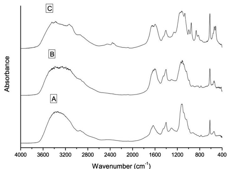
**Figure 4.** FT-IR spectra of the azo dye RR198 before (A) and after microaerophilic (B) and aerobic (C) treatments.
