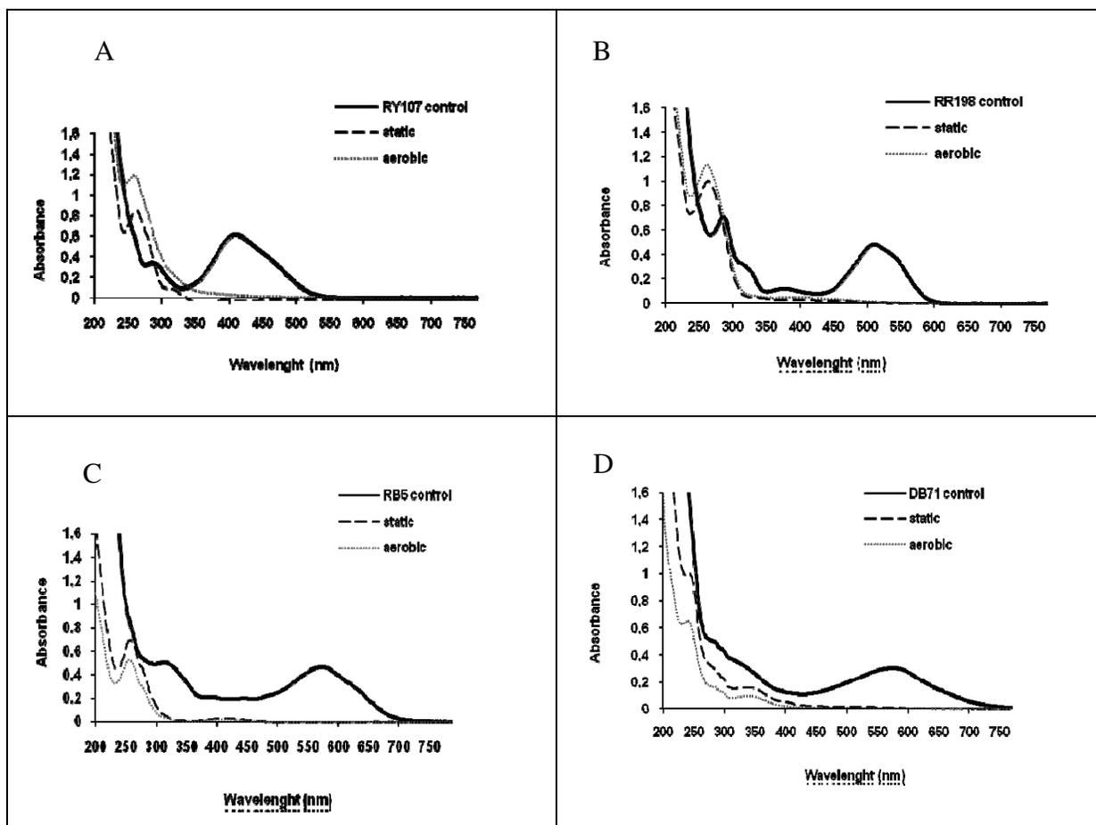
**Figure 3.** UV-Vis spectra of the azo dyes before (straight line) and after microaerophilic (dashed line) and aerobic (dotted line) treatments - A: RY107; B: RR198; C: RB5; D: DB71.
