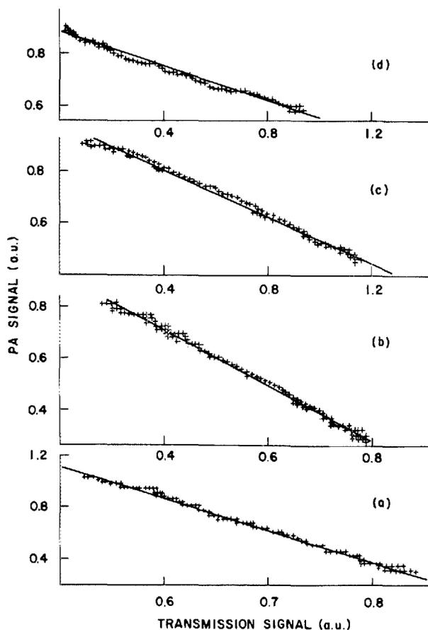
FIG. 4. Correlation between photoacoustic and transmission spectra for the various  $\text{MnO}_2$ -PE samples (labels correspond to those in Table I).
