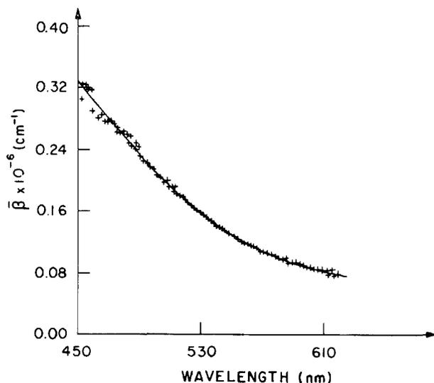
FIG. 5. The absorption coefficient for the new composite: manganese dioxide surface impregnated polyethylene ( $\text{MnO}_2\text{-PE}$ ).
