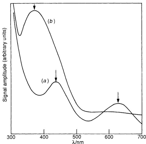
Fig. 1 PAS spectra of chromium in crystalline zeolitic chromosilicates, (a) ligand field bands of Cr<sup>III</sup>, (b) charge transfer band of Cr<sup>VI</sup>
