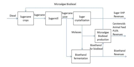
Figure 1. Block flow diagram of sugarcane refinery – microalgae biodiesel integration proposal
