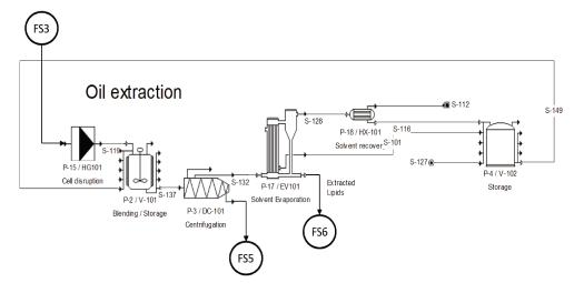
Figure 510. FS4 - PFD of oil extraction section
