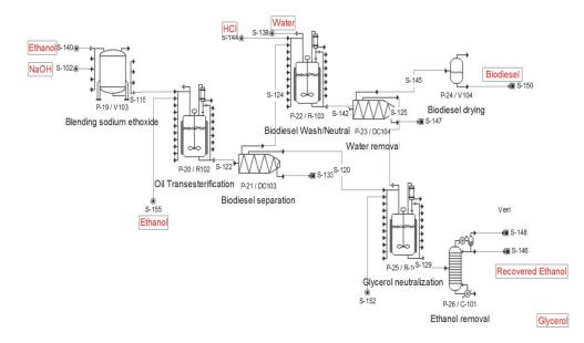
Figure 11. FS6 - PFD of biodiesel production section
