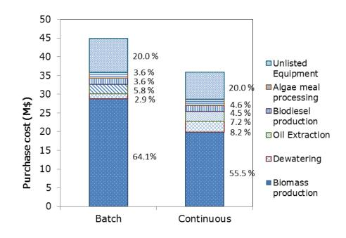
Figure 13. Equipment purchase costs for Batch and continuous mode
