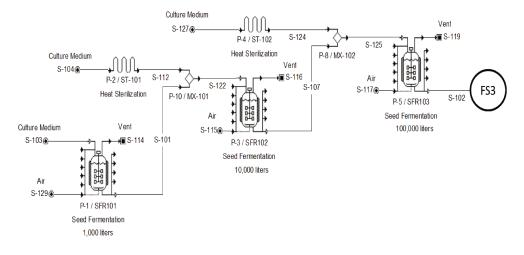
Figure 6. FS2 - Inoculum production configuration
