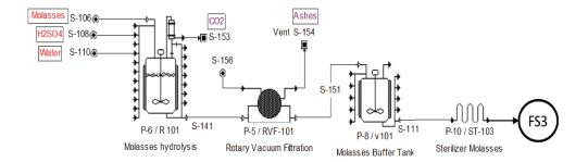
Figure 45. FS1 - Process flow design of molasses hydrolysis section
